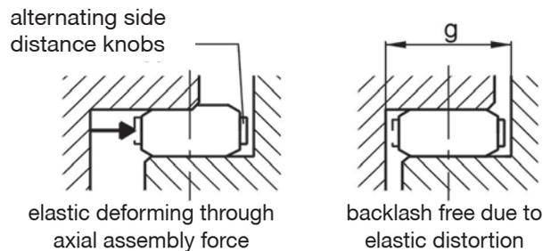
**Admissible seat clearance shaft / hub:** Series ESM-A: max 0,02 mm    Series EKM: min 0,01 mm/max 0,04 mm
