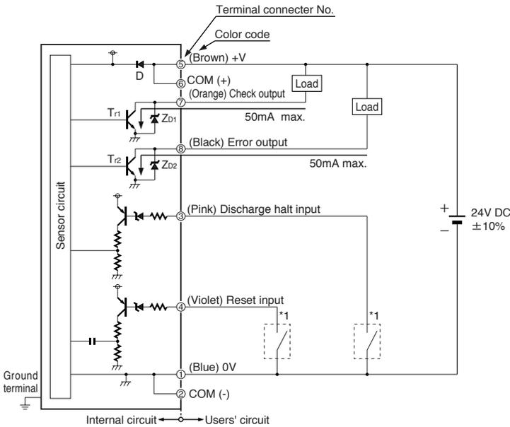
Symbols... D: Reverse supply polarity protection diode
